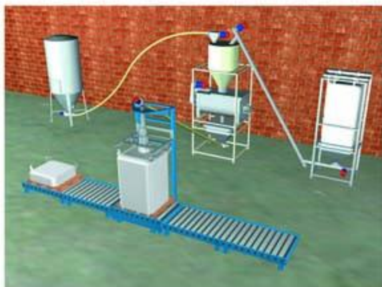
Automatic line for charging Bulk Bag on weigh cells located on rolling board
